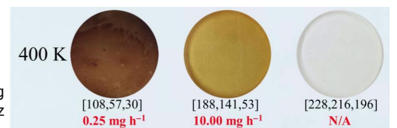
Fig 5 Hazes produced in a laboratory at conditions applicable to capability target atmospheres for the RCI from He et al. (2018)four. The metallicities from left to right are a hundred X, 1,000 X and 10,000 X leading to differing formation prices proven at backside in pink.
