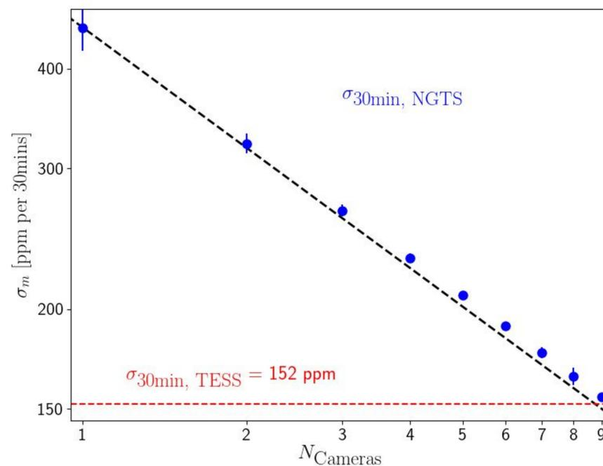
Figure 2: Improvement in photometric precision obtained with increasing number of telescopes used. The dashed lines give the best case theoretical improvement that would be obtained if the noise was 100% white noise (black) and the precision obtained by TESS for objects of similar magnitude (red)
