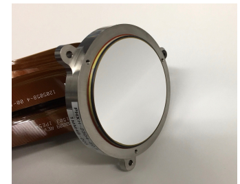
Xinetics 48 x 48 DM used in JPL's HCIT. Image Credit: J. Trauger (JPL)
