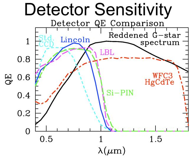
The spectrum of a typical reddened source star is compared to the QE curves of CCDs and Si-PIN detector arrays. The HgCdTe detectors developed for HST's WFC3 instrument can detect twice as many photons as the most IR sensitive Si detectors (CCDs or CMOS). MPF will employ 35 HgCdTe detectors. 3 filters: "clear" 600-1700nm, "visible" 600-900nm, and "IR" 1300-1700nm.
