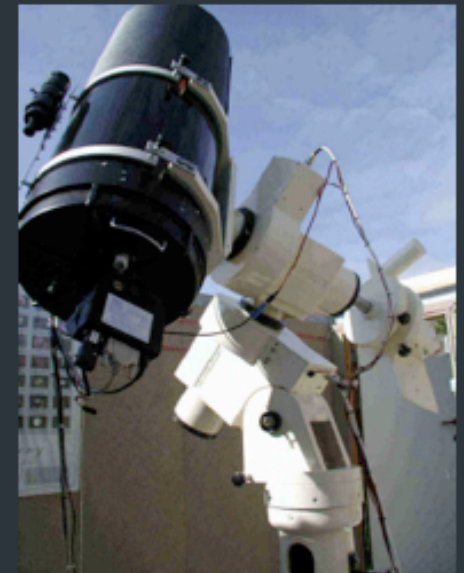
CBA Belgium Observatory features two CCD-equipped 0.35-m (14 Inch) Celestron Schmidt-Cassegrain telescopes on computerized mounts
