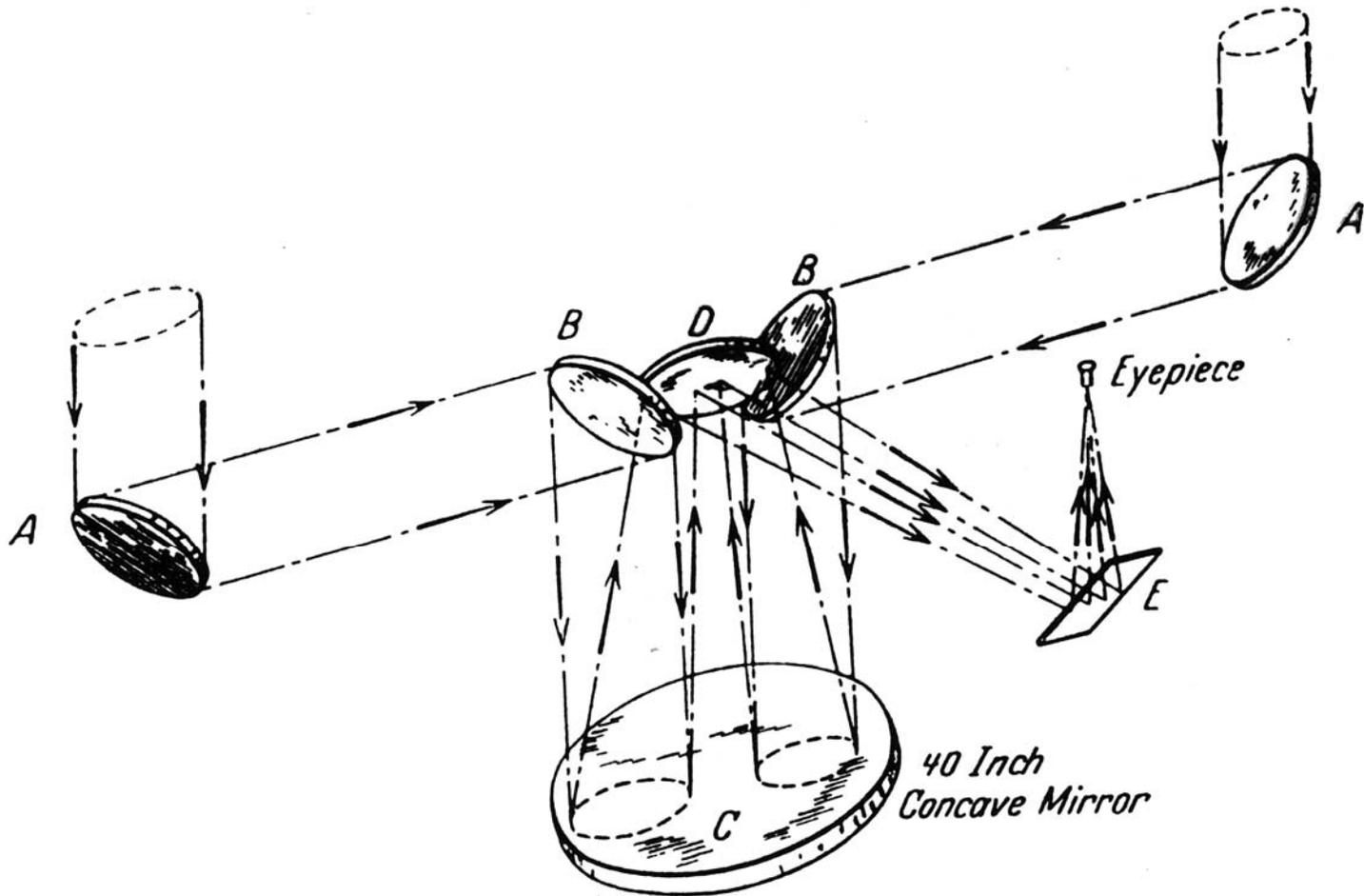
Abb. 8. Diagram of light path in 50 foot interferometer.
