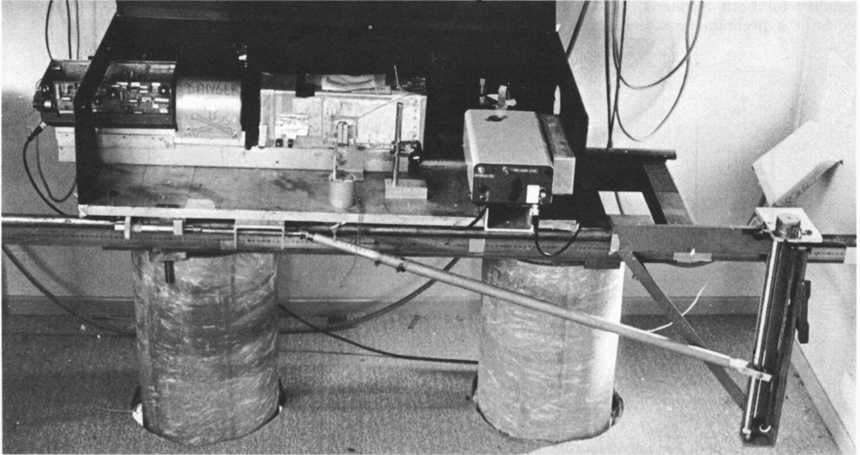
FIG. 3.—Central station, showing the optical table with its tracks, and the fringe-tracking mechanism which approximates the required cosine  $H$  displacement law. The concrete piers independent from the building are also visible, as well as the micrometer screw which allows for fine fringe tracking.
