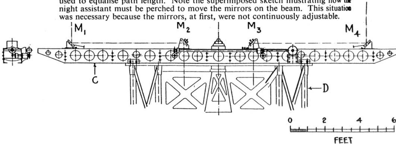
FIG. 2.—Diagram of 20-foot interferometer beam.  $M_1, M_2, M_3, M_4$ , mirrors;  $B, B$ , 10-inch channels;  $C$ , steel plate;  $E, E$ , screws to move outer mirrors;  $F$ , motor drive for screws;  $D$ , Cassegrain cage.
