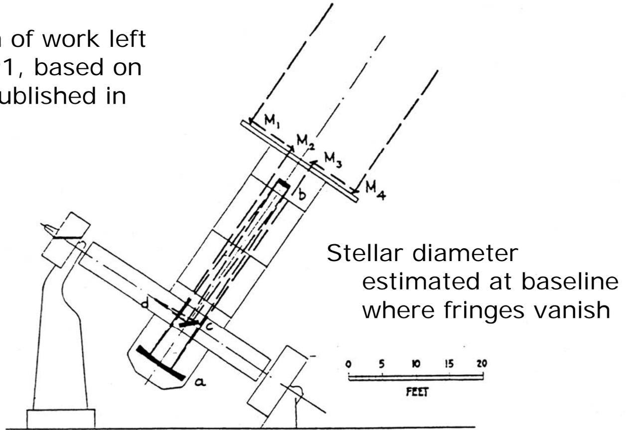
FIG. 1.—Diagram of optical path of interferometer pencils.  $M_1$ ,  $M_2$ ,  $M_3$ ,  $M_4$ , mirrors;  $a$ , 100-inch paraboloid;  $b$ , convex mirror;  $c$ , coude flat;  $d$ , focus.
