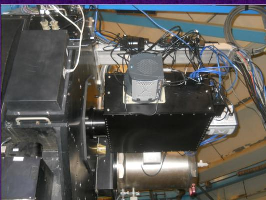
NESSI mounted on the WIYN 3.5-m telescope (black box with its two EMCCD imaging cameras sticking out). The silver cylinder behind and below is the WIYN Near-IR imager, WHIRC.
