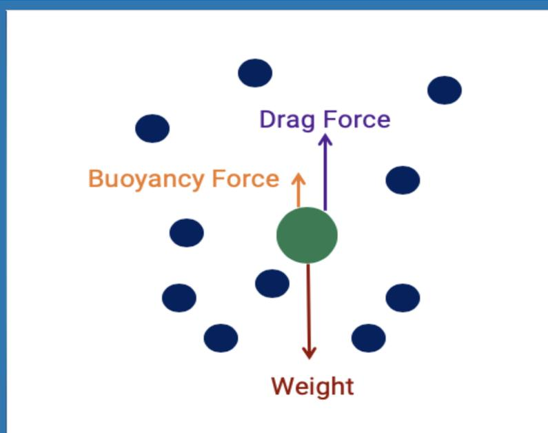
Figure 1: Force diagram showing the forces exerted on an oxygen atom (blue) due to its weight and the buoyancy and drag forces due to the escaping hydrogen (green). This force balance provides the basis of determining the crossover mass.
