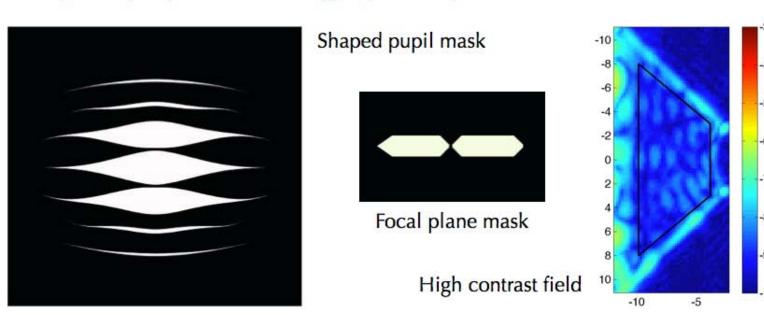
At left, the transmittance profile of a representative shaped pupil apodization (black indicates opaque, white indicates clear). At center, the corresponding "bowtie" image plane mask. This "Ripple 3" design achieved 2.4e-9 contrast in 10% bandwidth averaged over the 4-10  $\lambda/D$  dark field (outlined) on the HCIT. (Belikov et al. 2007)
