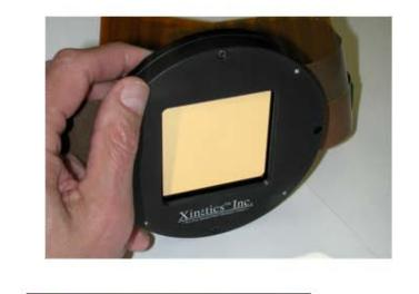
HCIT experiments have been carried out with Xinetics DMs. Fused silica facesheet is polished nominally to λ/100 rms. Surface figure (open loop) has been shown to be settable to 0.05 nm rms and stable to 0.01 nm rms over periods of 6 hours or more in a vacuum testbed environment. Protoflight qualification is in progress at JPL.
