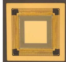
by Boston Micromachines (left) and IRIS-AO (right) can be configured with either continuous or segmented mirror facesheets. MEMS DMs are actively in use in all testbeds other than HCIT.
