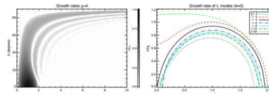
The figure in the left shows the growth rates as a function of  $q=k/k_{\text{BH}}$  and the angle  $\theta$  between the wavevector of disturbances and the vertical axis. The strongest destabilization is for pure  $k_z$  modes. The resonances correspond to the weaker de-stabilization at intermediate  $\theta$ , and exist for smaller wavelengths.
