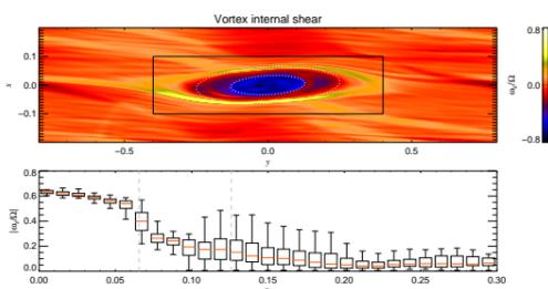
The vortex core is well enclosed by an ellipse of aspect ratio  $\chi=4$ . We measure the vertical vorticity in the mid-plane of the simulation against the elliptical radius, in the grid points boxed by the thin black line. The conclusion is that the vortex core has a Gaussian angular velocity profile, thus close to uniform rotation at the center.
