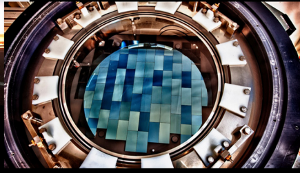
The 520 megapixel Dark Energy Camera (DECam)
