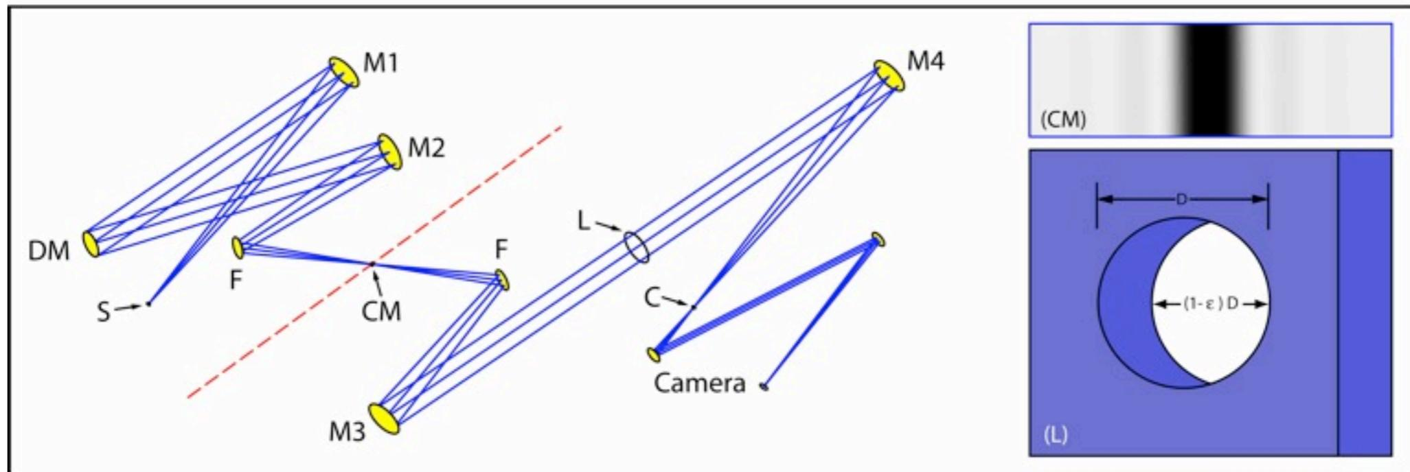
*Elements of the HCIT Lyot coronagraph: the light source (S) is a 5 micron pinhole illuminated by light relayed from a fiber; four identical off-axis paraboloidal mirrors (M1, 2, 3, 4); two flat fold mirrors (F), the band-limited focal plane mask (CM); the Lyot mask (L); the high-contrast coronagraph field appears at (C); and the CCD camera with a pair of OAP mirrors for 3x magnification.*
