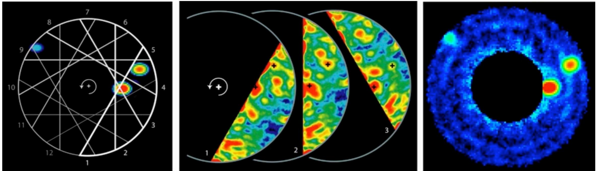
*Simulations of coronagraph data processing, with laboratory data, illustrate one method to distinguish Earth-like planets from the glare of the central star.*
