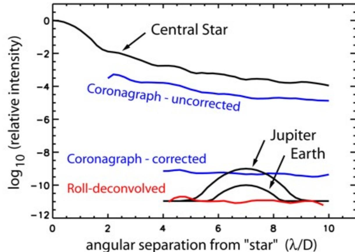
Comparison of azimuthally averaged PSFs of (a) the star, with focal plane mask offset and Lyot stop in place; (b) the coronagraph field with all DM actuators set to equal voltages; (c) the coronagraph with DM set for a dark half-field; and (d) the result of simulated roll deconvolution with the set of 480 consecutive coronagraph images. PSFs of a nominal Earth and Jupiter are also indicated.
