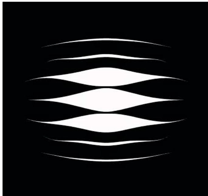
At left, the transmittance profile of a representative shaped pupil apodization (black indicates opaque). This “Ripple 3” design achieved:  $IWA = 4 \lambda/D$ , 10% bandwidth,  $C = 2.4 \text{ e-}9$  on the HCIT (Belikov et al. 2007).
