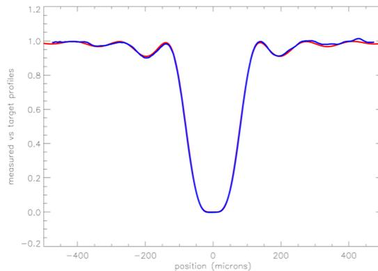
Comparison of the prescribed transmittance profile with the measured profile of the mask pictured at left. Desired profile is the red curve, the measured profile is the blue curve.
