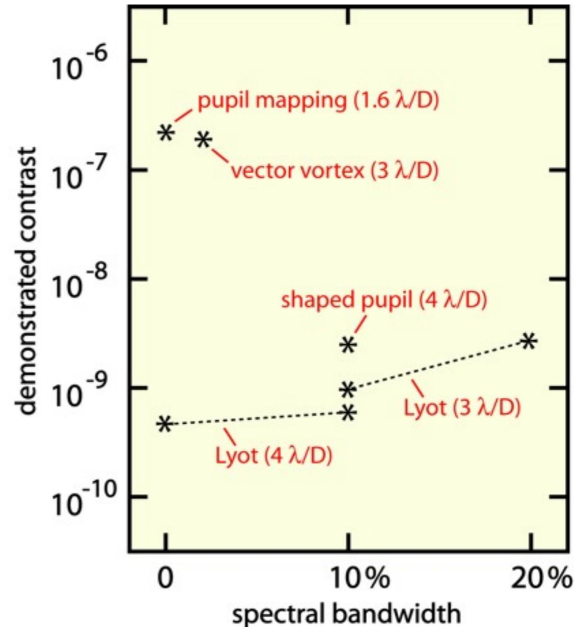
*The four major coronagraph types perform starlight rejection with combinations of phase and amplitude elements placed in focal and pupil planes. Best demonstrated laboratory contrast to date (July 2009) are indicated at right. Significant improvements are expected in the coming year as an outcome of active laboratory developments with well-understood technologies.*
