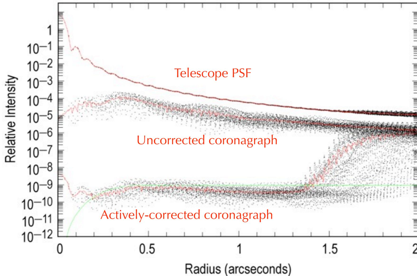
*Plotted are the point spread functions (PSFs) of a 1.8 meter telescope, coronagraph, and coronagraph with active wavefront correction. Instrument contrast is better than  $1e-9$  with an inner working angle of 0.25 arcsec for broadband (20%) visible light.*
