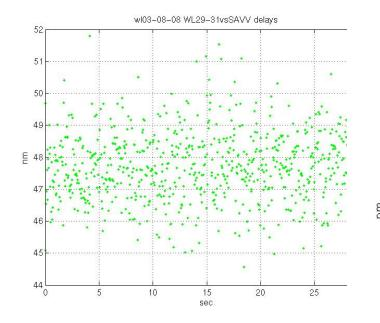
Testbed data @ 25 hz (40msec) at high freq, the noise looks like Gaussian white noise
