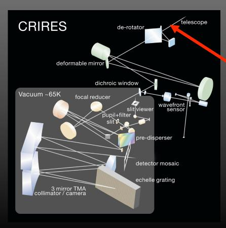
gas cell goes here to enable calibration of each observation
