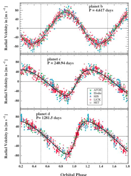
RV gives us K, RV amplitude P, period  $\epsilon$ , eccentricity  $\omega$ , periastron  $\angle$ T<sub>0</sub>, time of  $\omega$
