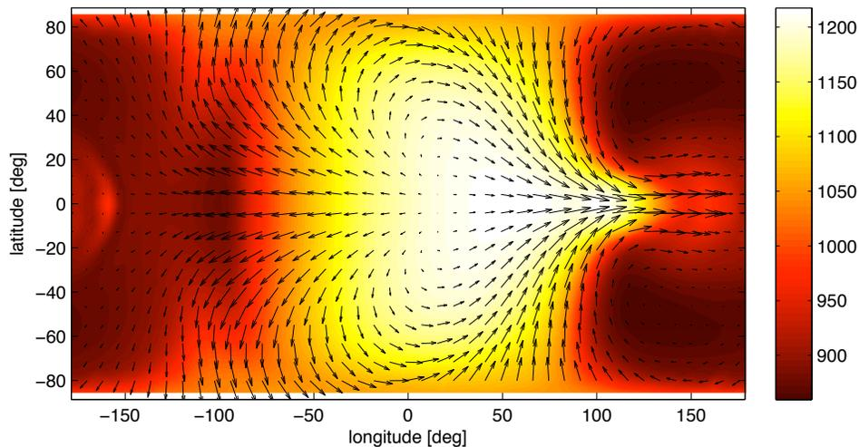
Notice the striking similarity between this flow pattern and the analytic theory. The Kelvin and Rossby wave structures are obvious, and they produce the necessary velocity tilts to generate superrotation. Once the model has spun up, superrotation indeed results:
